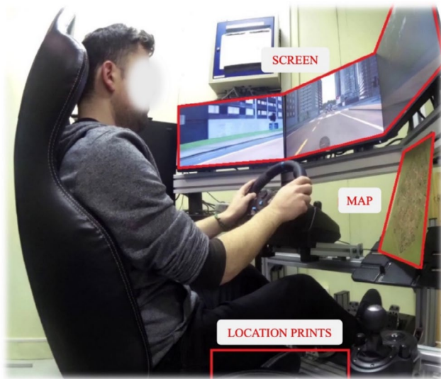
FIGURE 1 | Driving simulation setup and representation of the three main visual areas of interest (AOIs).
